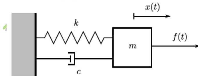
**Figure 1.46:** structure masse-ressort
