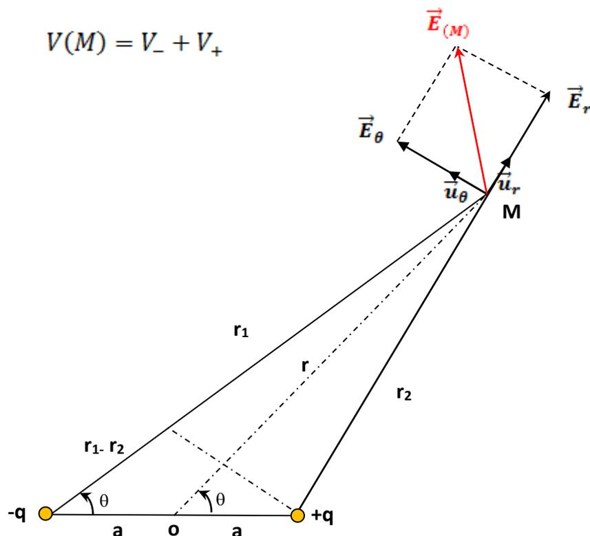
$$V(M) = k \frac{-q}{r_1} + k \frac{+q}{r_2} = k \left( \frac{q}{r_2} - \frac{q}{r_1} \right) = kq \left( \frac{1}{r_2} - \frac{1}{r_1} \right)$$
