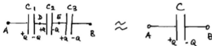
$$V_A - V_B = (V_A - V_D) + (V_D - V_E) + (V_E - V_B) = \frac{Q}{C_1} + \frac{Q}{C_2} + \frac{Q}{C_3} = \frac{Q}{C}$$
