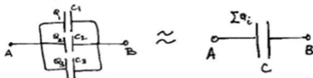
$$V_A - V_B = \frac{Q_1}{C_1} = \frac{Q_2}{C_2} = \frac{Q_3}{C_3} = \frac{Q}{C} = \frac{Q}{C_1 + C_2 + C_3}$$
