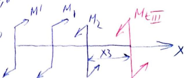
$$\alpha_3 = \int_0^{0,8} \frac{M_{t\overline{II}} dx_3}{GI_0} = \int_0^{0,8} \frac{(M_1 + M' - M_2) dx_3}{GI_0} = \left. \frac{(M_1 + M' - M_2)x_3}{GI_0} \right|_0^{0,8}$$
