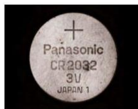
A battery with shallow dents under standard coaxial illumination
