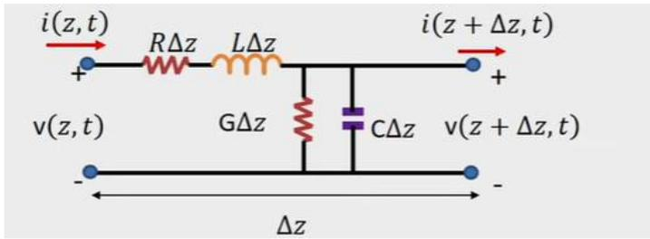
$$v(z, t) - R\Delta z i(z, t) - L\Delta z \frac{\partial i(z, t)}{\partial t} - v(z + \Delta z, t) = 0$$
