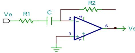
$$Z = R2 // Z_C = \frac{\frac{R2}{jC\omega}}{R2 + \frac{1}{jC\omega}} = \frac{R2}{1 + jR2C\omega} \quad Z_C = R1 + \frac{1}{jC\omega} = \frac{1 + jR1C\omega}{jC\omega}$$
