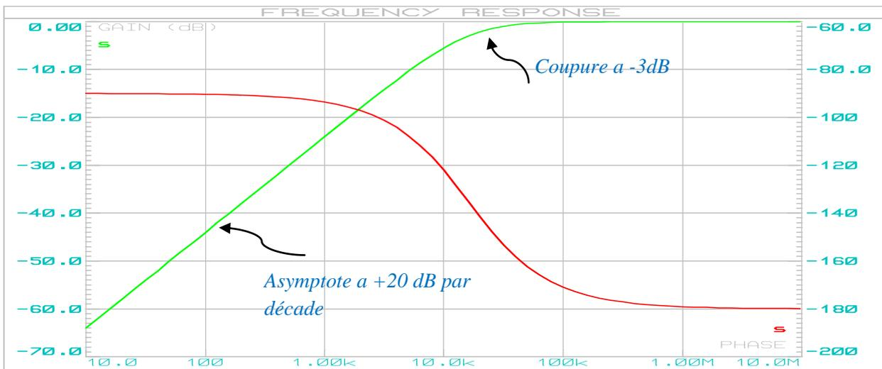
$$|F(j\omega)| = \left| k \frac{j \frac{\omega}{\omega_0}}{1 + \frac{j\omega}{\omega_0}} \right| = \frac{\left| k j \frac{\omega}{\omega_0} \right|}{\left| 1 + \frac{j\omega}{\omega_0} \right|}$$
