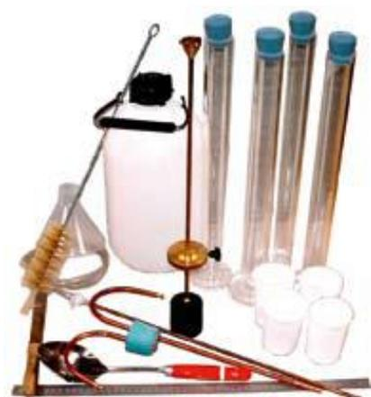
APPAREILLAGE POUR ESSAI D'EQUIVALENT DE SABLE
